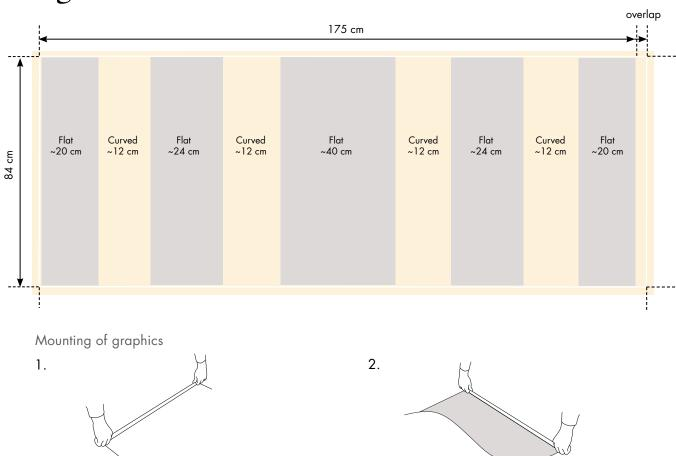
Mount first part of the Vecro/magentic tape along the vertical edge of the panel. This shall be on the BACK side of the panel.
