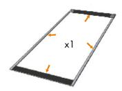
Front Panel: Start by mounting the provided top and bottom strips, according mage above. Then carefully mount the magnetic tape along the sides of the panels.
