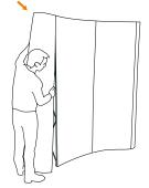
The side panels are assembled last in the same way as the others. Manually help curve the panels to easier get them in place (depending on print material).
