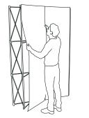
Mount the front panels according image above. They are easily guided and attached with the magnets in the top corners of each panel.
