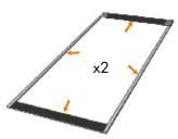
Front Panels: Start by mounting the provided top and bottom strips, according mage above. Then carefully mount the magnetic tape along the sides of the panels. Side Panels: Mount the top corner strips on the side panels. Assembly the magnetic tapes in the same way as in previous step.
