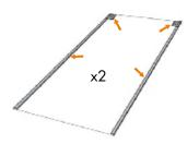
Side Panels: Mount the top corner strips on the side panels. Assembly the magnetic tapes in the same way as in previous step.
