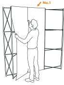
Mount the front panels according image above. They are easily guided and attached with the magnets in the top corners of each panel. For best result always start with the centre panel.
