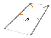
Side Panels: Mount the top corner strips on the side panels. Assembly the magnetic tapes in the same way as in previous step.
