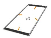
Front Panels: Start by mounting the provided top and bottom strips, according mage above. Then carefully mount the magnetic tape along the sides of the panels.
