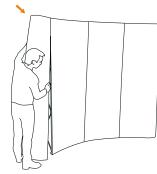
The side panels are assembled last in the same way as the others. Manually help curve the panels to easier get them in place (depending on print material).
